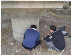
Fig. 5. Hardness test of pier
